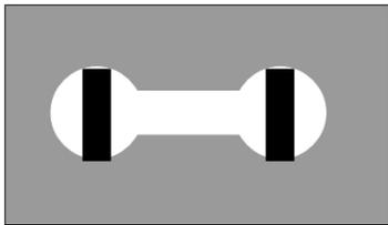
The addition of black stripes in each circular portion of the dumb bell at right angles to the shaft signifies that aeroplanes and gliders taking off or landing must do so on a runway but that movement on the ground is not confined to hard surfaces.
