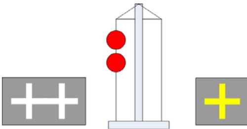
A double white cross and/or two red balls suspended from a mast one above the other signify that glider flying is taking place at the aerodrome.
