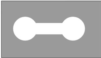
A white dumb bell signifies that movements of aeroplanes and gliders shall be confined to paved, metalled or similar hard surfaces.
